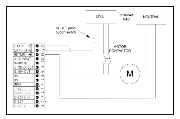
Note: Push button switch needs to be held down for 2-3 seconds to activate the RESET function.
