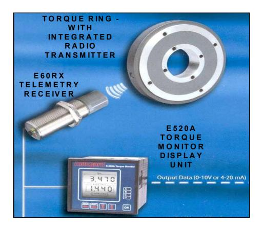
The Torque Ring is typically of the form as shown above. The outer flange is bolted to one part of the drive train, and the inner flange to the other part. Strain gauges measure the torque being transmitted through the Torque Ring and this data is converted via the integral battery powered circuitry into a radio signal.
