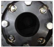
Standard on the MS series, the interlocking flange arrangement utilizes the fasteners in clearance holes to allow components to shift slightly in the event of a disc pack failure and act as a simple pin & bush coupling.
