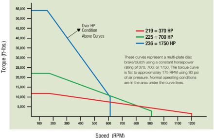
Horsepower Curves 219, 225, 236 AquaMaKKs (Standard Linings)
