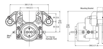
The Twiflex VCS-FL disc brake caliper comprises a single spring module forming the 'active' side of this floating unit and is available for use where space is limited or to accommodate axial disc float of ±6mm.
