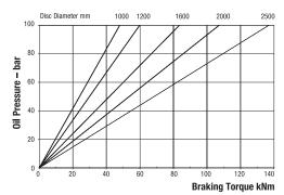
Maximum Pressure 100 bar Maximum Braking Force = 118kN @ 100 bar Weight of caliper (2 modules) - 80kg Volume displacement per 1mm stroke at both pads = 31ml
