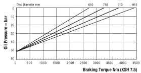
Maximum Braking Force XSH 7.5: 11.2kN Minimum Pressure for full retraction: 63 bar Weight of caliper and thruster - 13.62kg
