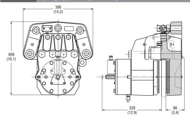
The Twiflex VKSD-FL disc brake caliper comprises a single spring module forming the 'active' side of this floating unit and is available for use where space is limited or to accommodate axial disc float of ±6mm.
