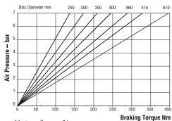
Maximum Pressure 7 bar Maximum Braking Force = 1.44kN @ 7 bar Weight of caliper and thruster - 2.5kg Weight thruster only - 1.0g Volume displacement of thruster at full stroke = 150ml
