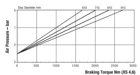
Maximum Braking Force XS 4.6: 6.8kN Minimum Pressure for full retraction: 3 bar Weight of caliper and thruster - 13.72kg Weight of thruster only - 4.5kg Volume displacement of thruster at full retraction = 1.19 I
