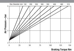
Maximum Pressure = 7 bar Minimum Pressure for full retraction = 4.3 bar Maximum Braking Force = 0.6kN
