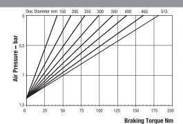
Maximum Pressure = 7 bar Minimum Pressure for full retraction = 1.75 bar Maximum Braking Force = 0.76kN
