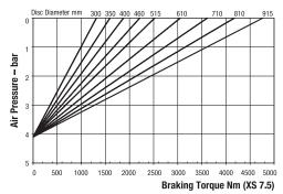
Minimum Pressure for full retraction: 5.5 bar Maximum Braking Force XS 7.5: 11.2kN Weight of caliper and thruster - 11.9kg
