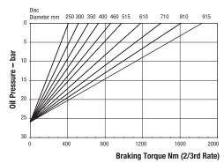
Minimum Pressure for full retraction 33 bar Maximum Braking Force 2/3rd rate: 4.3kN Weight of MR caliper and thruster - 10.5kg Weight of MR2 caliper and thruster - 11kg
