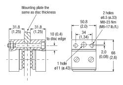
The Twiflex T2 disc brake caliper is split caliper design suitable for use with a minimum disc thickness of 5mm. The modules are mounted each side of a central mounting plate of the same thickness as the brake disc. Minimum disc diameter is 120mm. Alternatively, the brake may be side-mounted with a spacer equal to the disc thickness between the two halves.
