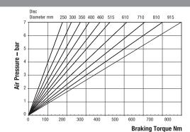
Maximum Pressure 7 bar Maximum Braking Force = 1.9kN @ 7 bar Weight of MR caliper and thruster - 6.8kg
