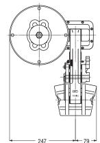
Maximum Braking Force = 6kN Weight of caliper and actuator - 17.9kg
