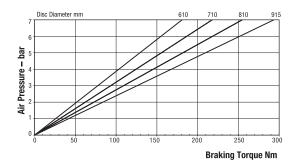
Maximum Pressure 7 bar Maximum Braking Force = 0.74kN @ 7 bar Weight of caliper and thruster - 9.56kg
