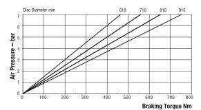
Maximum Pressure 7 bar Maximum Braking Force = 1.9kN @ 7 bar Weight of caliper and thruster - 9.52kg
