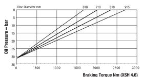
Maximum Braking Force XSH 4.6: 6.8kN Minimum Pressure for full retraction: 40 bar Weight of caliper and thruster - 13.22kg
