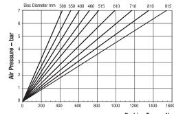
Maximum Pressure 7 bar Maximum Braking Force = 3.6kN @ 7 bar Weight of caliper and thruster - 8.15kg Braking Torque Nm Weight thruster only - 1.15kg Volume displacement of thruster at full stroke = 150ml
