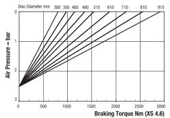
Minimum Pressure for full retraction: 3.1 bar Maximum Braking Force XS 4.6: 6.8kN Weight of caliper and thruster - 11.5kg
