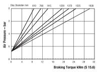
Maximum Braking Force S 15.6: 36kN Minimum Pressure for full retraction: 8.4 bar Weight of calipper and thruster - 49kg Weight of thruster only - 15kg Volume displacement of thruster at full retraction = 1.3 l
