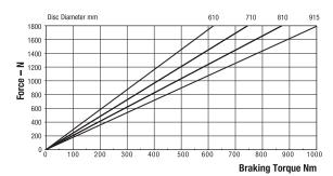
Weight of caliper and hand wheel assembly - 10.52kg Weight of hand wheel assembly only - 1.3kg Maximum Braking Force = 2.68kN
