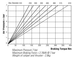
Weight of caliper and thruster - 2.8kg Weight of thruster only - 1.3kg Volume displacement of thruster at full stroke = 300ml
