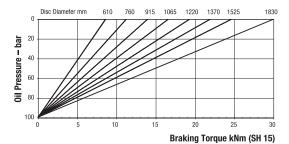
Maximum Braking Force SH 15: 35kN Minimum Pressure for full retraction: 120 bar Weight of caliper and thruster - 53kg Weight of thruster only - 19kg Volume displacement of thruster at full retraction = 56ml
