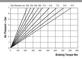
Maximum Pressure 7 bar Maximum Braking Force = 1.9kN @ 7 bar Weight of caliper and thruster - 7.3kg
