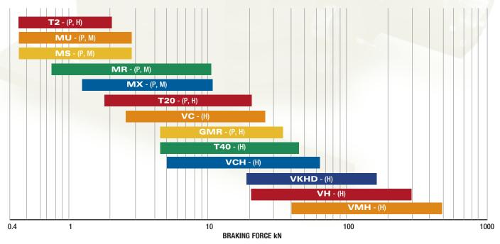
\*It should be noted that the braking forces shown are for a single caliper only and multiple calipers may often be used on a disc, with available space being the typical limitation.
