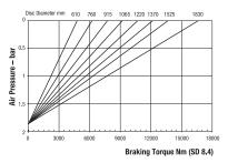
Maximum Braking Force SD 8.4: 19.5kN Minimum Pressure for full retraction: 2.4 bar Weight of caliper and thruster - 52.2kg Weight of thruster only - 18.2kg Volume displacement of thruster at full retraction = 2.5 l
