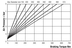
Maximum Pressure = 7 bar Minimum Pressure for full retraction = 6.2bar Maximum Braking Force = 2.6kN
