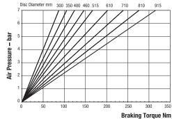
Maximum Pressure 7 bar Maximum Braking Force = 0.74kN @ 7 bar Weight of caliper and thruster - 7.34kg Weight of thruster only - 0.34kg Volume displacement of thruster at full stroke = 25ml
