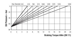
Maximum Braking Force SH 11: 25kN Minimum Pressure for full retraction: 92 bar Weight of caliper and thruster - 51.2kg Weight of thruster only - 17.2kg Volume displacement of thruster at full retraction = 56ml
