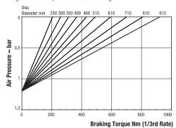
Minimum Pressure for full retraction: 1.7 bar Maximum Braking Force 1/3rd rate: 2.2kN Weight of MR caliper and thruster - 10.0kg Weight of MR2 caliper and thruster - 10.5kg
