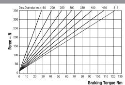
Weight of caliper and thruster - 1.9kg Weight of hand wheel assembly only - 1.15kg Maximum Braking Force = 0.51kN
