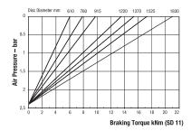
Maximum Braking Force SD 11: 25kN Minimum Pressure for full retraction: 3.3 bar Weight of caliper and thruster - 53.2kg Weight of thruster only - 19.2kg Volume displacement of thruster at full retraction = 2.5 l
