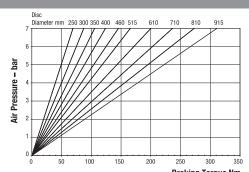
Maximum Pressure 7 bar Maximum Braking Force = 0.74kN @ 7 bar Weight of MR caliper and thruster - 6.84kg Weight of MR2 caliper and thruster - 7.34kg **Braking Torque Nm**Weight of thruster only - 0.34kg
