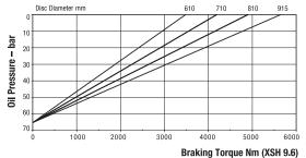
Maximum Braking Force XSH 9.6: 14.3kN Minimum Pressure for full retraction: 82 bar Weight of caliper and thruster - 13.82kg
