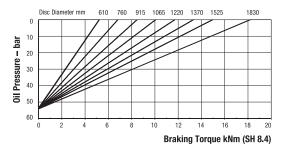
Maximum Braking Force SH 8.4: 19.5kN Minimum Pressure for full retraction: 65 bar Weight of caliper and thruster - 50.2kg Weight of thruster only - 16.2kg Volume displacement of thruster at full retraction = 56ml
