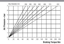
Maximum Pressure 7 bar Maximum Braking Force = 0.76kN @ 7 bar Weight of caliper and thruster - 1.89kg
