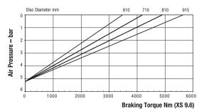
Maximum Braking Force XS 9.6: 14.3kN Minimum Pressure for full retraction: 6.5 bar Weight of caliper and thruster - 14.32kg
