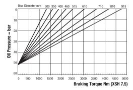
Minimum Pressure for full retraction: 65 bar Maximum Braking Force XSH 7.5: 11.2kN Weight of caliper and thruster - 11.4kg
