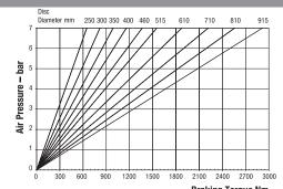
Maximum Pressure 7 bar Maximum Braking Force = 6.9kN @ 7 bar Weight of MR caliper and thruster - 7.82kg Weight of MR2 caliper and thruster - 8.32kg Braking Torque Nm Weight of thruster only - 1.32kg Volume displacement of thruster at full stroke = 300
