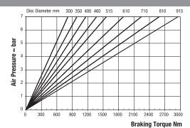
Maximum Pressure 7 bar Maximum Braking Force = 6.9kN @ 7 bar Weight of caliper and thruster - 8.32kg Weight of thruster only - 1.32kg Volume displacement of thruster at full stroke = 300ml
