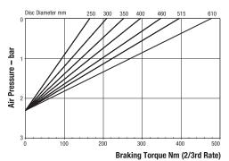
Maximum Braking Force 2/3rd rate: 1.74kN Minimum Pressure for full retraction: 3.3 bar Weight of caliper and thruster - 4.9kg
