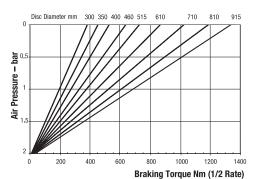
Minimum Pressure for full retraction: 2.5 bar Maximum Braking Force 1/2 rate: 3.2kN Weight of caliper and thruster - 10.5kg
