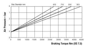
Maximum Braking Force XS 7.5: 11.2kN Minimum Pressure for full retraction: 5 bar Weight of caliper and thruster - 14.12kg Weight of thruster only - 4.9kg Volume displacement of thruster at full retraction = 1.19 I
