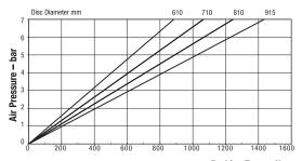
Maximum Pressure 7 bar Maximum Braking Force = 3.6kN @ 7 bar Weight of caliper and thruster - 10.37kg
