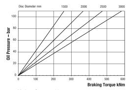
Maximum Pressure 110 bar Maximum Braking Force = 433kN @ 110 bar Weight of caliper ( 2 modules ) - 580kg Volume displacement per 1mm stroke at both pads = 101.5ml
