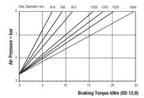
Maximum Braking Force SD 12.9: 30kN Minimum Pressure for full retraction: 3.8 bar Weight of caliper and thruster - 54kg Weight of thruster only - 20kg Volume displacement of thruster at full retraction = 2.5 l
