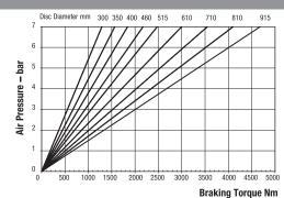
Maximum Pressure 7 bar Maximum Braking Force = 11kN @ 7 bar Weight of caliper and thruster - 9.06kg Weight of thruster only - 2.06kg Volume displacement of thruster at full stroke = 426ml
