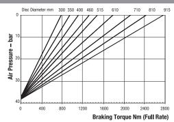
Minimum Pressure for full retraction: 50 bar Maximum Braking Force full rate: 6.4kN Weight of caliper and thruster - 11kg
