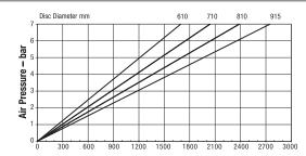
Maximum Pressure 7 bar Maximum Braking Force = 6.9kN @ 7 bar Weight of caliper and thruster - 10.54kg
