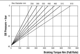
Maximum Braking Force full rate: 2.6kN Minimum Pressure for full retraction: 50 bar Weight of caliper and thruster - 5.5kg Weight of thruster only - 4kg Volume displacement of thruster at 4mm retraction = 5ml
