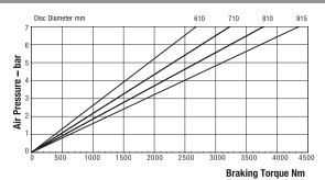
Maximum Pressure 7 bar Maximum Braking Force = 11kN @ 7 bar Weight of caliper and thruster - 11.28kg Weight of thruster only - 2.06kg Volume displacement of thruster at full stroke = 426ml
