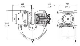
The Twiflex VS Mk2 disc brake caliper is comprised of two modules secured between U-shaped top and bottom mounting plates by tie rods.
