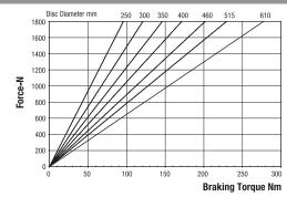
Maximum Braking Force = 1.01kN Weight of caliper and hand wheel Retraction pressures where shown are calculated and may vary depending on spring tolerance. assembly - 2.53kg
