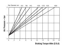
Maximum Braking Force S 8.4: 19.5kN Minimum Pressure for full retraction: 4.8 bar Weight of caliper and thruster - 46.2kg Weight of thruster only - 12.2kg Volume displacement of thruster at full retraction = 1.3 l
