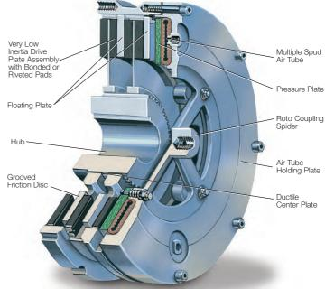
keep power demands below the allowed maximum. Heat generated by controlled slipping or high cycle rate operation is dissipated by the centrifugal blower design of these units. These clutches and brakes interface well with automated controls through simple air and/or electric circuits.
