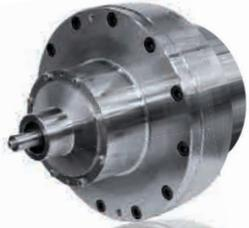
The double stage input uses the reliable, high load Cyclo stage on the scroll side – i.e. where high torque loads occur. This Cyclo stage has also featured in the ZS – Cyclo Line series. Combination with a planetary stage enables exceptionally high reduction rates of up to 348/1. High differential speeds can also be achieved.
